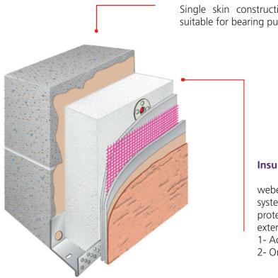
Single skin construction in a thickness suitable for bearing purposes only.
