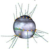
Schematic shows cement particle with polymer backbone and the long lateral chains linked to it.
