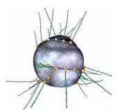
Schematic shows cement polymer particle with backbone and the long lateral chains linked to it.
