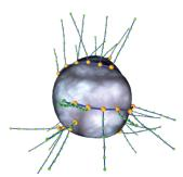
Schematic shows cement polymer particle with backbone and the lateral chains linked to it.
