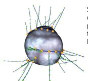
shows Schematic cement particle with polymer backbone and the long lateral chains linked to it.
