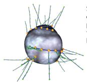
shows Schematic cement particle with polymer backbone and the long lateral chains linked to it.
