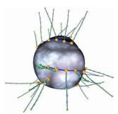
Schematic shows cement particle with lateral chains linked to it.
