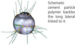
shows cement particle with polymer backbone and the long lateral chains
