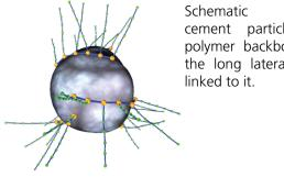
shows cement particle with polymer backbone and the long lateral chains
