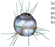
Schematic shows cement particle with polymer backbone and the long lateral chains linked to it.
