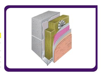
Position the profiles (rails having convenient space depending on the thickness of the boards), and fix them well by drilling to allow the passage of the dowels. The space between each dowels must be around 30 cm.
