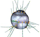
Schematic shows cement particle with polymer backbone and the long lateral chains linked to it.
