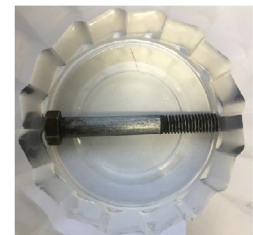
steel rod with water +1% Admix PCI
